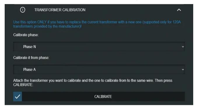
These calibration instructions and the Transformer Calibration function can also be used to recalibrate the phase A / B or C measuring transformers, e.g. after replacement.
