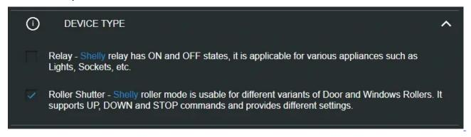
Relay - Configure Shelly Device as a 2-circuit relay, two separately switchable relay outputs O1 / O2
