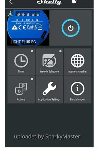
The Shelly is now successfully included in the app "Shelly Cloud" and can be operated and controlled remotely with the mobile phone or a pad while the cloud is activated.
