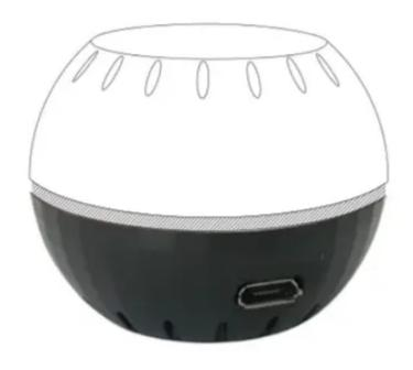
With this Shelly H & T accessory, you can power your H & T via a micro USB cable with any 5V power adapter.
